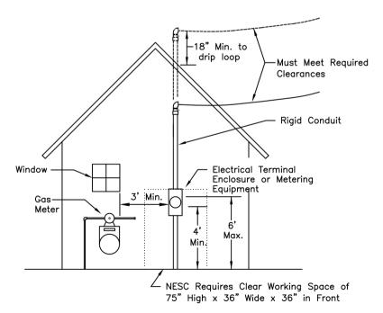
3-foot minimum clear working space required between electric meter and gas meter.
