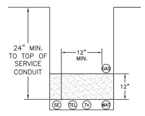
MAINTAIN 12"HORIZONTAL SEPERATION & 12" VERTICAL SEPERATION BETWEEN GAS & SE CONDUIT
